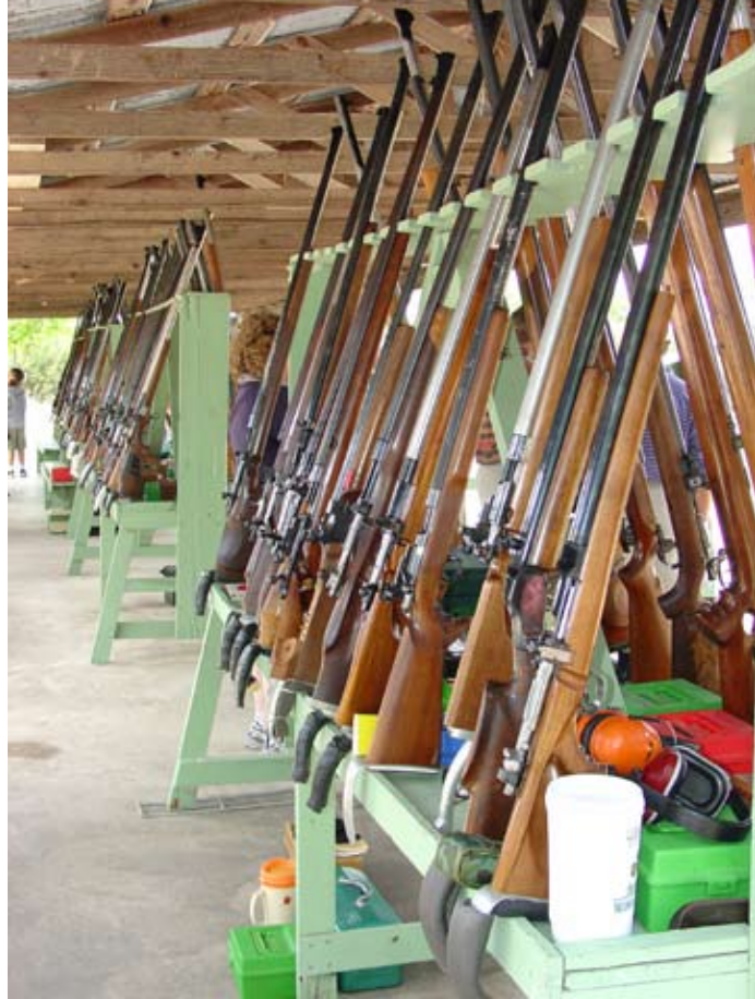
Row upon Row of the some of the most accurate rifles in the area. The guns must meet various requirements to be entered in the contest. The rear sight must have a slit that is not too narrow, or not closed, which would make it a peep sight; the front sight must be a post, not a ball. The front post is blackened with a sooty flame.
